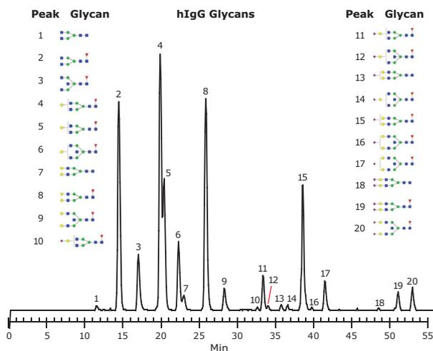
A sample of human IgG glycans was analyzed on a BIOshell™ Glycan HPLC column resulting in the identification of 20 distinct peaks. Glycans were identified by mass spectrometry, which was coupled in line with the HPLC-fluorescence detector system. Excellent separation as well as symmetrical peak shape can be observed in the chromatogram.
