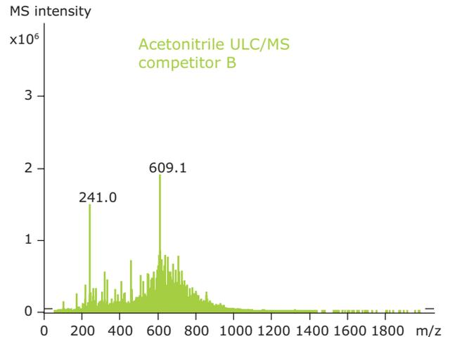
Mass spectra displaying the results of the reserpine test of different acetonitrile qualities from MilliporeSigma and two alternative competitors.
