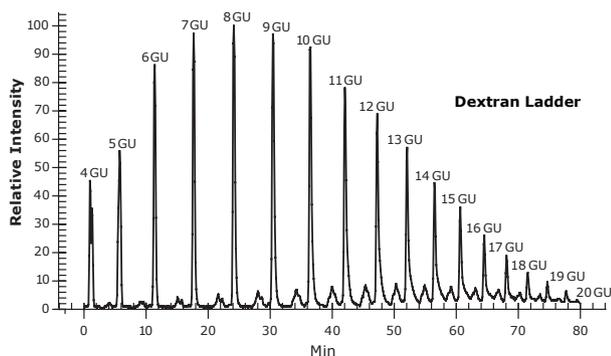
The dextran ladder is used as an external standard for the analysis of glycans by HILIC mode HPLC after fluorescent labeling. When analyzed on the BIOshell™ Glycan HPLC column, this standard gives a characteristic ladder profile from monomeric glucose to a 20-mer glucose oligosaccharide. This ladder provides calibration reference points that can aid in identifying more complex glycans based upon retention characteristics.
