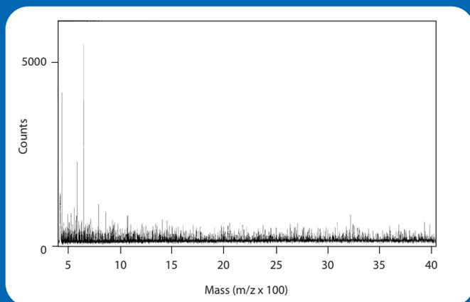
ZipTip® pipette tips increase sensitivity of mass spectrometric analysis. MALDI MS spectra of a tryptic peptide digest from an in-gel 2D digest. The top spectrum represents a contaminated sample prior to sample clean-up. The lower spectrum represents the sample after treatment with a ZipTip® C18 tip prior to MALDI-ToF MS analysis.
